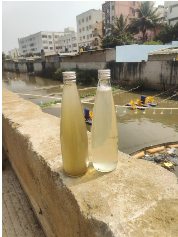
Before and After Treatment Samples of the Sewage Water at the Nalla
